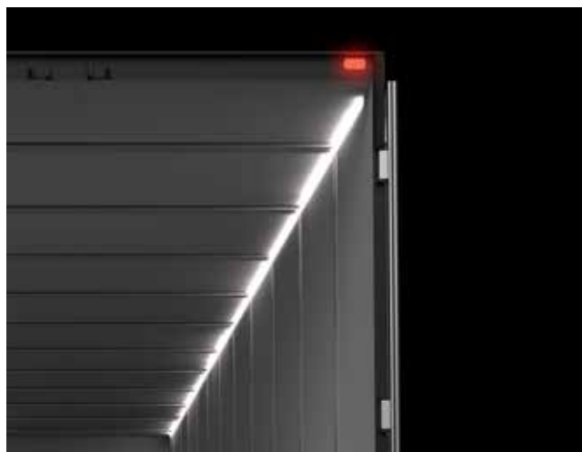
Interior lighting for truck trailers / mounting with corner profile
