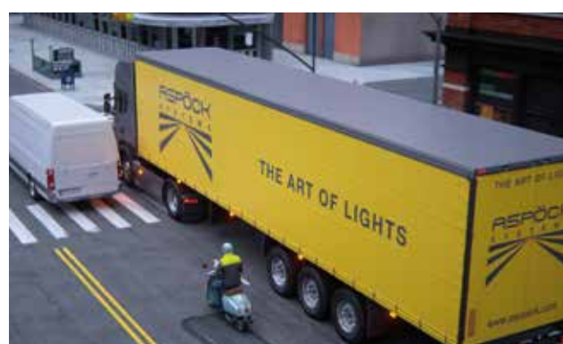
Flashing side marker lamps along the truck trailer are an important safety factor for other road users.
